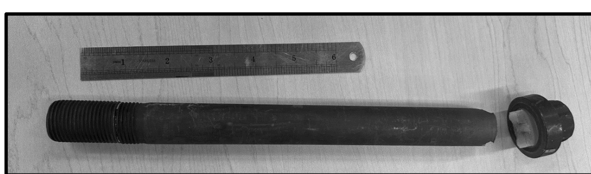
Figure 5. Failed Damper Bolt
