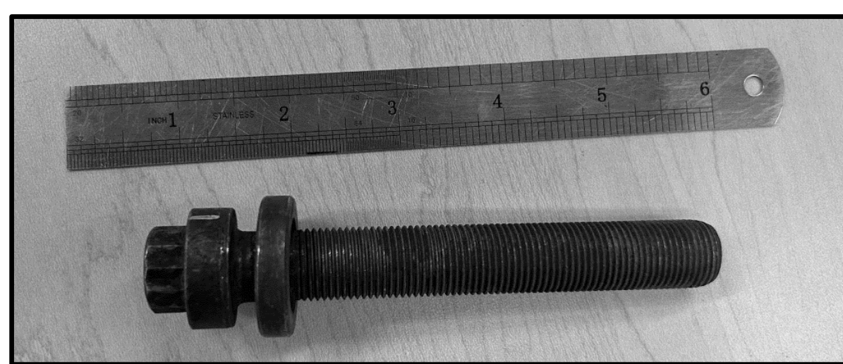
Figure 4. Intact Counterweight Bolt
